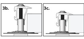
3a. 4. Exercise care when threading the Male Portion of the Stand-Off into the clamp to avoid crossthreading 5. 6.
